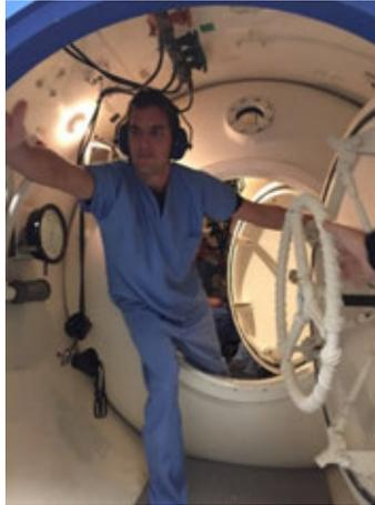
*Shutting the chamber door before pressurization with students to an equivalent pressure of 130ft sea water. (Credit: NOAA/Stephen Matadobra)*
