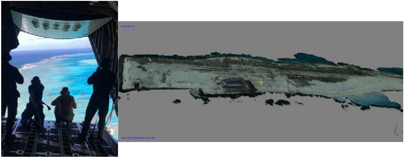
Above: LTJG Terril Efird (second from left) takes a series of images from the USCG C-130 used to create a 3D image (right), which can be used to quantify storm damage. (Credits: Keo Lopes, top; Terril Efird, images; rendering Keo Lopes, bottom).
