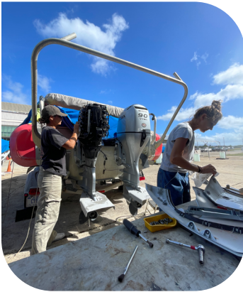
(Left) PNMS Field Team members conduct an engine deep clean as a part of its end of year service schedule. Photo: Alexa Gonzalez. (Right) PNMS Field Team conducts an annual lift test to test the structural integrity of the small boat hull, lifting points, and lifting straps. Photo: Jennifer McCullough.
