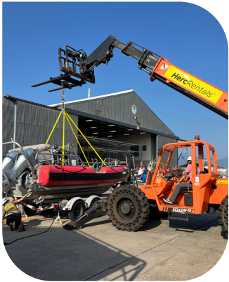
(Left) PNMS Field Team members conduct an engine deep clean as a part of its end of year service schedule. Photo: Alexa Gonzalez. (Right) PNMS Field Team conducts an annual lift test to test the structural integrity of the small boat hull, lifting points, and lifting straps. Photo: Jennifer McCullough.
